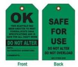
Green tags are indicators that the scaffold has passed inspection and that the competent person has cleared the scaffold for safe use. These tags should be attached to the scaffold at each access point.
